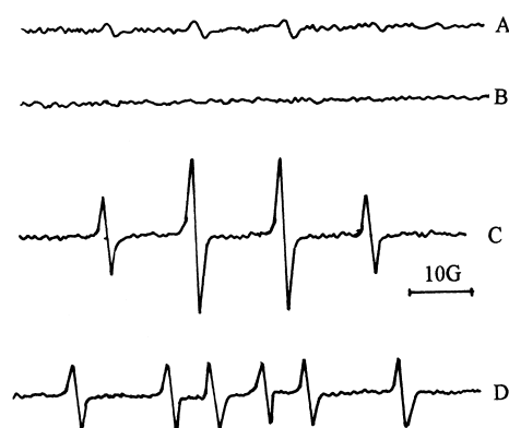
Fig. 5. EPR spectra of DMPO-hydroxyl radical adduct produced from irradiation of an oxygen-saturated buffer solution of Cys-HB (0.1 mM, pH 7.4) and DMPO (50 mM). (A) sample prepared in the daylight, (B) In the absence of Cys-HB or oxygen or irradiation. (C) On irradiation for 2 min, (D) As in (C) but in the presence of \text{CH}_3\text{CH}_2\text{OH} and the solution was incubated in the dark for 2 min after irradiation. (Instrumental settings – microwave power, 8 mW; modulation amplitude, 1 G; scan range, 200 G; receiver gain, 1 \times 10^4 ).
